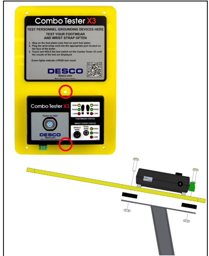
Figure 6. Securing the Combo Tester X3 to the pedestal
